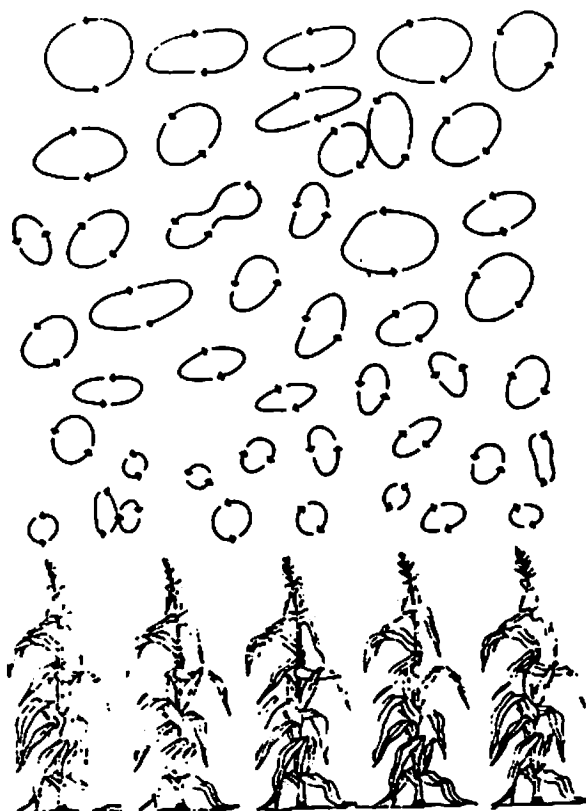
Figure 9.2 Schematic illustration of small packets or eddies of air swirling about in the turbulent region above vegetation. The eddies, which tend to increase in size with height, carry all molecules they contain more or less as a unit. They are continuously changing size -- breaking up, or coalescing with other eddies -- making their actual size somewhat hypothetical.
